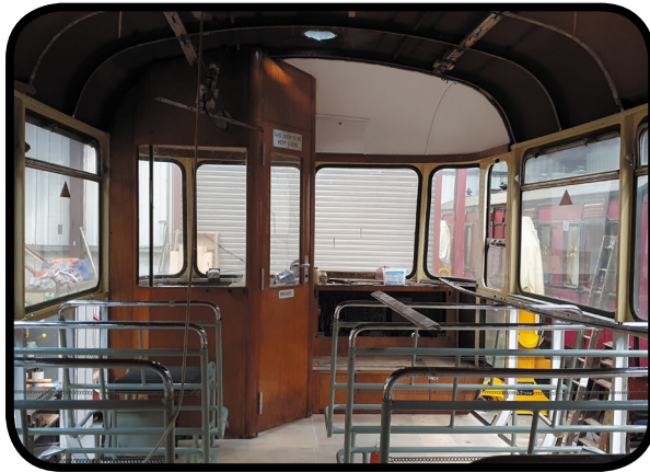
DRB Keighley end floor and seat restoration - Photo: Richard Jones
