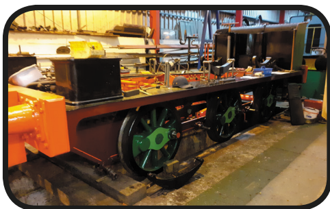
Sir Berkeley back on its wheels with the lining started on the frames and the 2 tone wheels.
