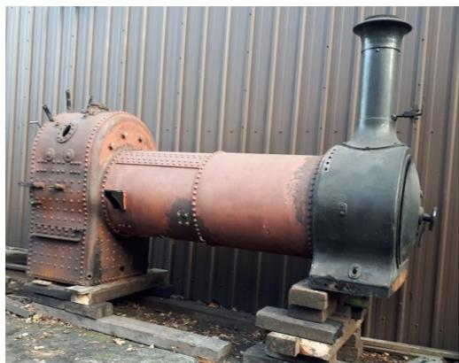
My accompanying photograph shows the boiler standing in Moor Road Yard. It should be noted that, although a modern boiler (built in 2005) it has been riveted, rather than welded as would be normal practice these days. This was done to preserve the historic nature of the locomotive – this boiler is in fact more or less what Manning, Wardle would have had to build in later years. It can be compared with the original boiler (also at Moor Road) to see the engineering advances.
