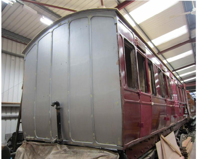
*The second photo dates from May 27<sup>th</sup> and shows an interrupted Stuart at work. Note the new ribs now in position. The compartment partitions and the roof planking followed in quick time.*
