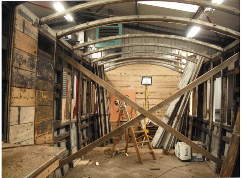
Stuart has also been busy making new beading and mouldings to replace those removed from this (Keighley) end in the distant past. Some replacement of mouldings is also taking place at the Oxenhope end of the coach.
