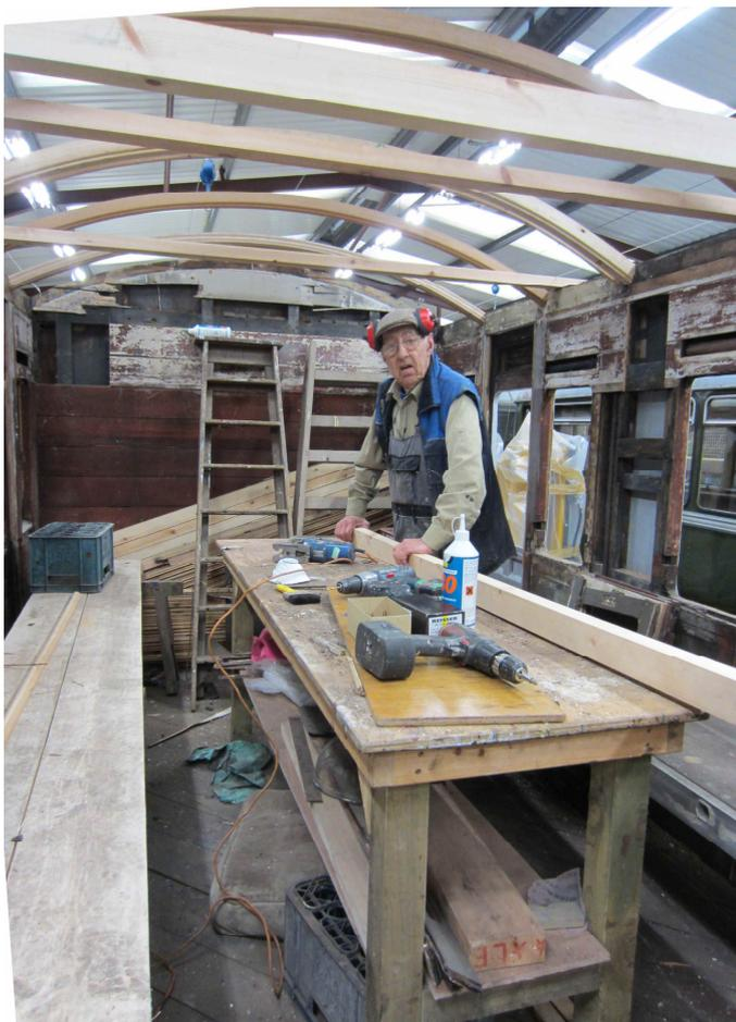
It is anticipated that the body will be lifted in the Autumn to enable Chris to overhaul the vehicle's brake rigging, suspension, draw gear and buffers. Allied with this part of the restoration will be the fitting of new end headstocks. The overhaul of the underframe is very important as a prelude to returning this late 18<sup>th</sup> Century vehicle to running condition for the 21<sup>st</sup> Century.
