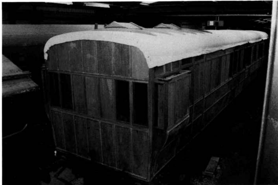
GNR 2856 with roof canvas in position but awaiting the gutter strips.
