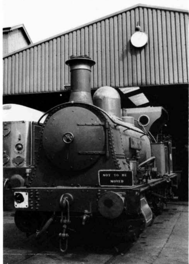
Not a cheerful sight – the 'Not To Be Moved' board and the removed buffer (to give access to the valve spindle) tell of Bellerophon's present problems
