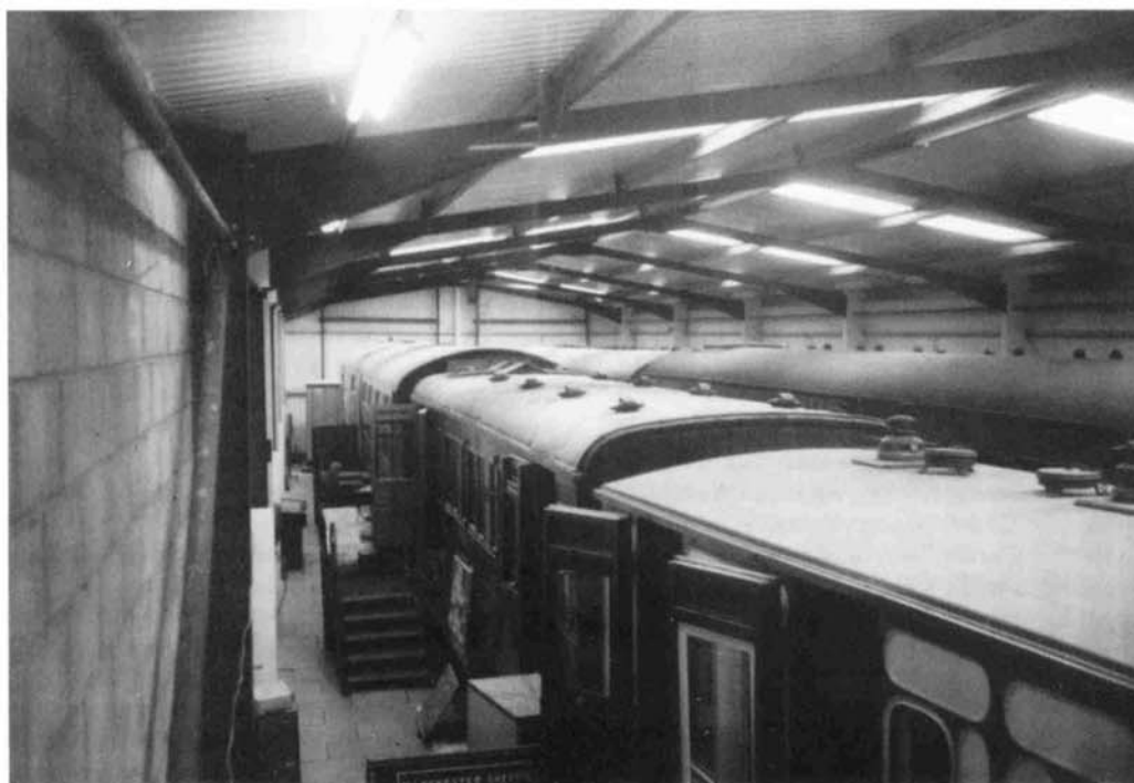
Coach roofs, seen from the Museum's upper storeroom before final completion of the 'sideways' extension. Note the non-authentic vents and the general absence of the correct roof furniture on our ECJS coach No. 143 (centre).
